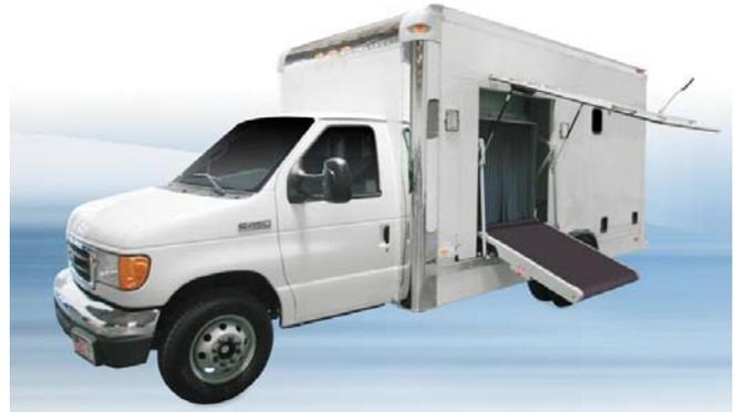
It is built into a Ford 450E van and includes a diesel power generator that supports all the utilities on board the vehicle, including the X-Ray machine and the air conditioning in the operator's compartment.
