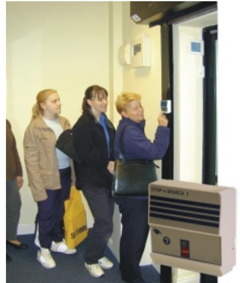
The principle of operation is the same for all units. WI-RSS-102 is usually activated on leaving the premises. The selection odds are set up on installation (5:1, 10:1, 20:1 and 50:1). It is completely random, virtually impossible to control the randomness of selection which is controlled electronically and does not create a guessable pattern.
