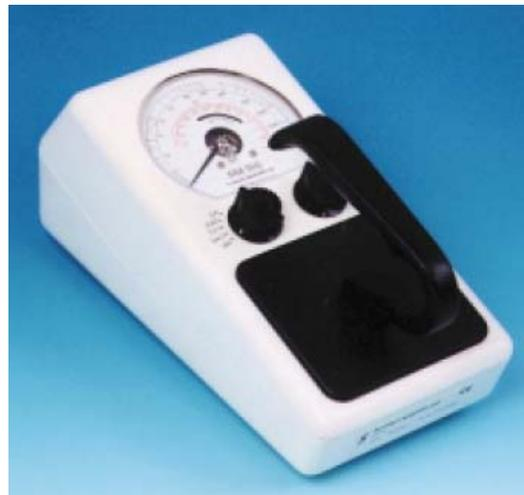
When the Geiger-Mueller probe position is selected a G-M overload circuit is activated which prevents the meter needle from falling back to a low level if the count rate from the G-M tube becomes so high that the pulse heights become attenuated. If this is switched on, an alarm tone is given and extra current is fed to the meter to hold it at full scale. This circuit is not active in the scintillation probe position.
