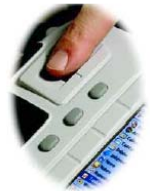
The 500dpi fingerprint sensor allows you to capture a high quality image to positively match identity.
